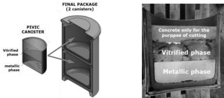
Fig. 3. PIVIC Package concept and vertical cut of a scale 1 canister produced with the first prototype of the project.
